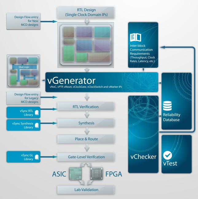
Synchronization failures are a common pitfall in multiple clock domain designs. These bugs are hard to fix, because the failures are often intermittent and hard to catch. Fixing such bugs in FPGA may take weeks of debugging, and they may be impossible to catch in ASIC prior to fabrication.
